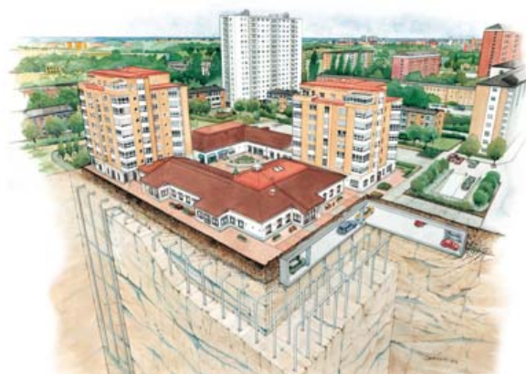
Figure 5: Borehole Thermal Energy Storage (BTES). Illustration: Geotec.
