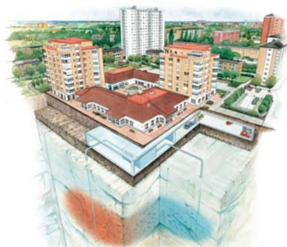
Figure 4: Aquifer Thermal Energy Storage (ATES). Illustration: Geotec.
